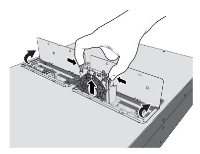
Figure 1. Replacing a System Fan
